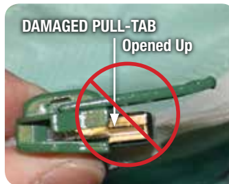
Zipper pull tabs are open/damaged and will not close the zippers.
