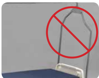
Canopy metal frame is bent or broken.
