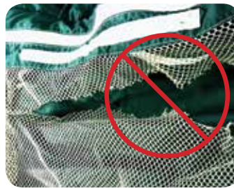
Canopy and netting have tears, holes, or abrasions.
